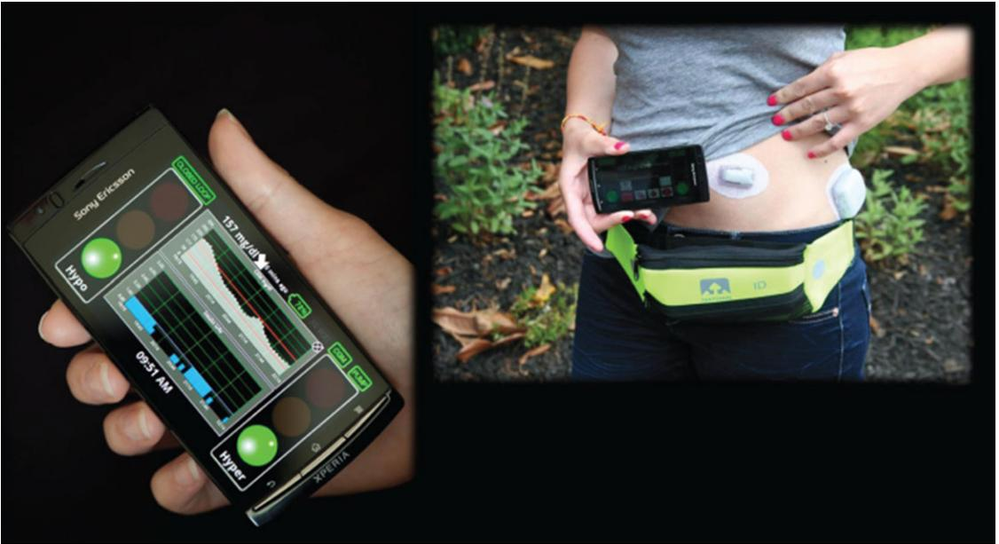
**Figure 4.** (Left) The DiAs smartphone used in recent UVA outpatient artificial pancreas studies with the closed-loop control algorithms operating on a smartphone rather than a laptop computer. (Right) A patient holding the DiAs smartphone next to the Dexcom CGM and Insulet insulin pump on her abdomen.<sup>45</sup>
